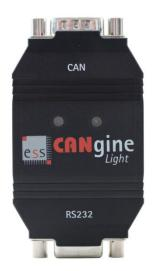
Sophisticated CAN message filtering allows to adapt the throughput to the baud rate of the serial link. Running the serial link with 230,4 kbit/s CANgine-generic can process up to 800 CAN frames per second (extended frame with 8 data byte) or 950 CAN frames per second (standard frame with 8 data byte).
